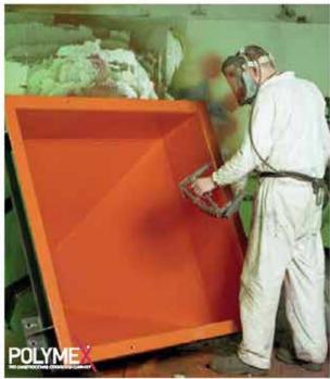
It is fire – resistant due to synthetic and silicone resin – based, antimony trioxide special resin additives. It is applied safely on surfaces contacting with high temperature. It is used in painting chimney, furnace and motor surfaces. It is necessary to clean newly applied surfaces thoroughly. If the second layer is applied over the first thin layer, a good result will be achieved. It is fire resistant up to 600 °C.
